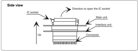
Figure 3.7 Opening and closing the IC socket
